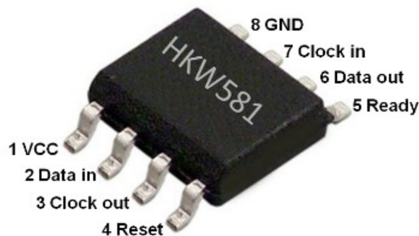
Figura 4: Pinout HKW581.
